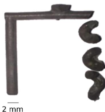
**Figure 4.** Part after demoulding. All samples showed an intact pillar, while the helix broke at the turning points.
