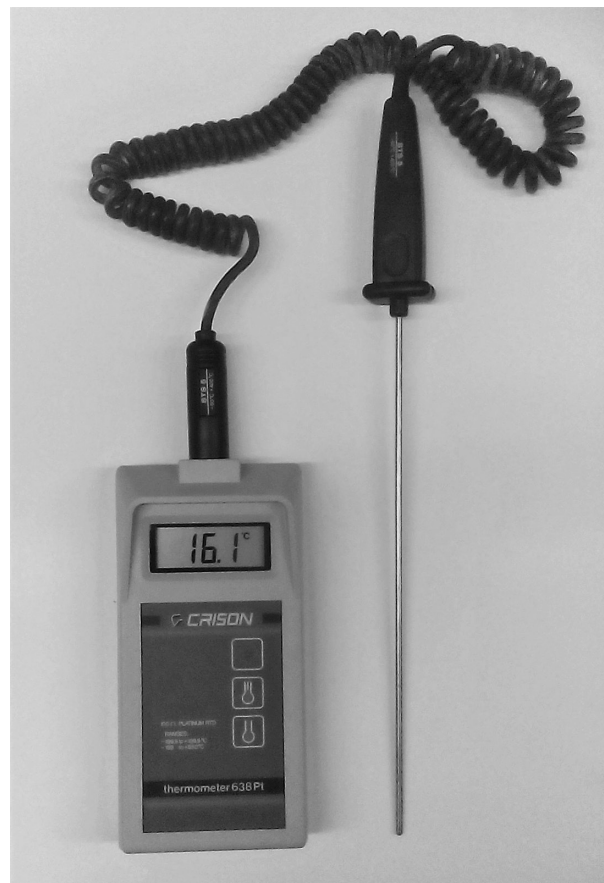
Fig. 1. The thermometer with a platinum probe used for measuring temperatures in the ventral vaginal fornix, 2–3 cm within the cervical canal, and 20 cm within the rectum.
