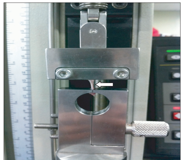
Fig. 3. The figure represents the biomechanical testing machine, Instron. Achilles tendon (arrow) was securely held with clamps and the lesion site was midway between the clamps.
