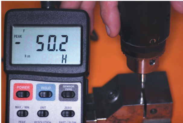
Figure 4- The digital torque meter showing the maximum torque required for loosening the screw
