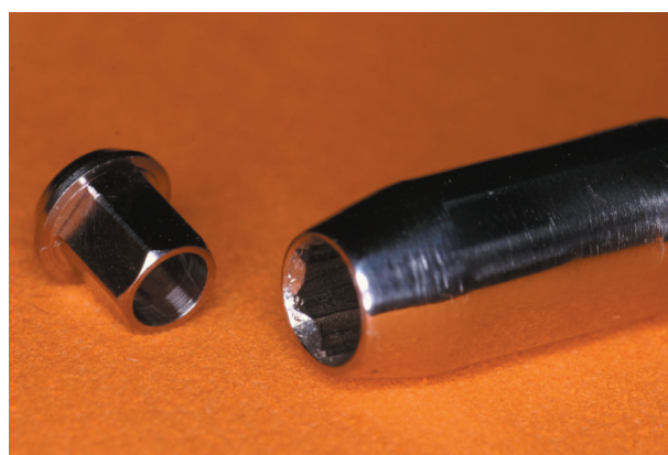
Figure 2- One of the ends of the custom-made wrench that fits onto the hexagonal abutment for loosening the screw
