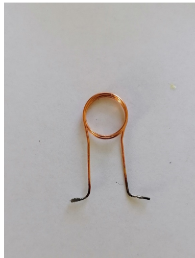
Figure 8. The appearance of the L1 inductor of the receiving coil.
