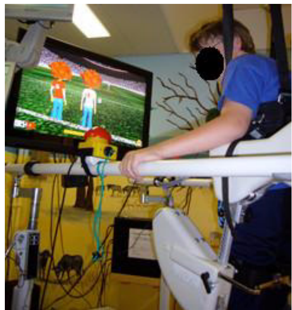
Figure 1 Robotic assisted gait training (RAGT). Child on the pediatric Lokomat with the display presented to the subjects during VR Soccer condition.
