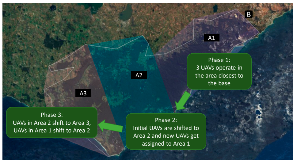
Figure 3. Mission concept illustrating the Unmanned Aerial Vehicles (UAVs) bounding strategy.
