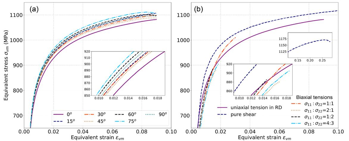
**Figure 5.** Flow stress curves of (a) uniaxial tension (UT) in different directions and (b) pure shear and biaxial tension with different stress ratios.  $\sigma_{11} : \sigma_{22}$  represents the stress ratio of the normal stresses in RD and TD.
