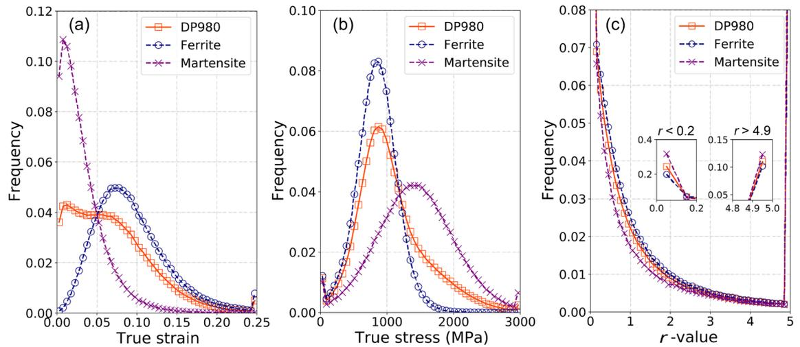
**Figure 11.** The histograms of the frequency distribution of true strain (bin size 0.005), true stress (bin size 60 MPa), and  $r$ -value (bin size 0.1) of the DP-RVE and the separated F-RVE and M-RVE. The RVE was subjected to uniaxial tension in RD at the specific plastic work of 60 MPa. The true stress and true strain correspond to the components in tensile direction.
