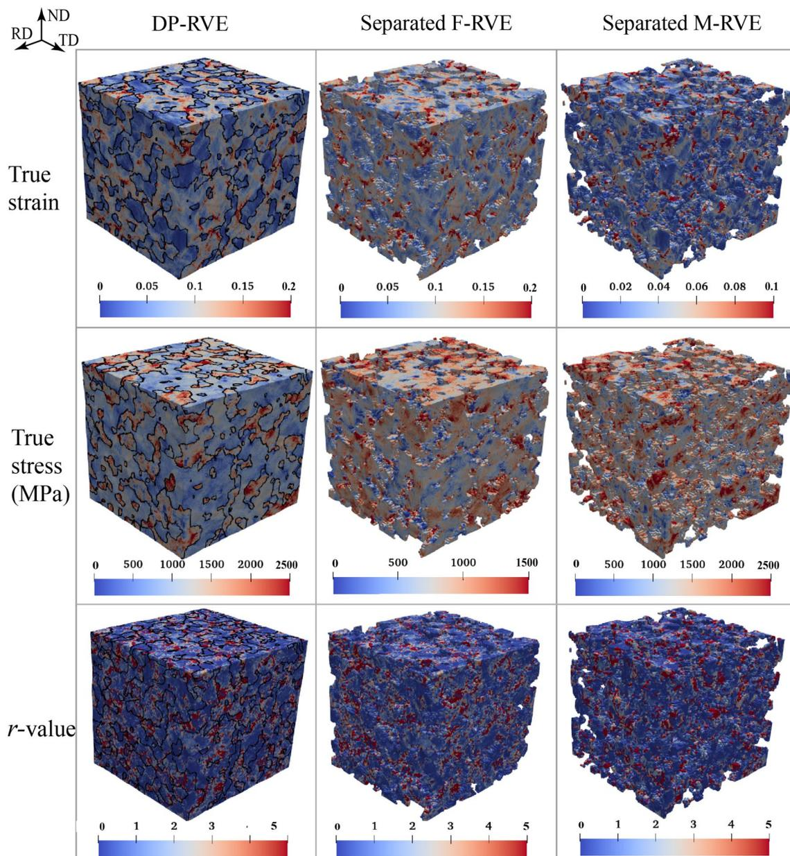
**Figure 10.** The contour maps of the true strain, true stress, and  $r$ -value of the DP-RVE and the separated M-RVE and F-RVE after the uniaxial tension in RD to the specific plastic work of 60 MPa. The true stress and true strain correspond to the components in the tensile direction.
