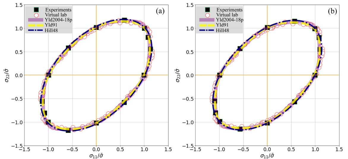
**Figure 6.** Yield loci ( $\sigma_{12} = 0$ ) of the DP980 sheet outlined by the experimental stress points (solid squares) of different loading conditions, enclosed by 60 random stress points (open circles) generated by the VL, and predicted by the calibrated yield functions (lines); the equivalent deformation stage with the specific plastic work of 3 MPa (a) and 8 MPa (b).  $\bar{\sigma}$  denotes the uniaxial tensile stress in RD obtained from the virtual tests.
