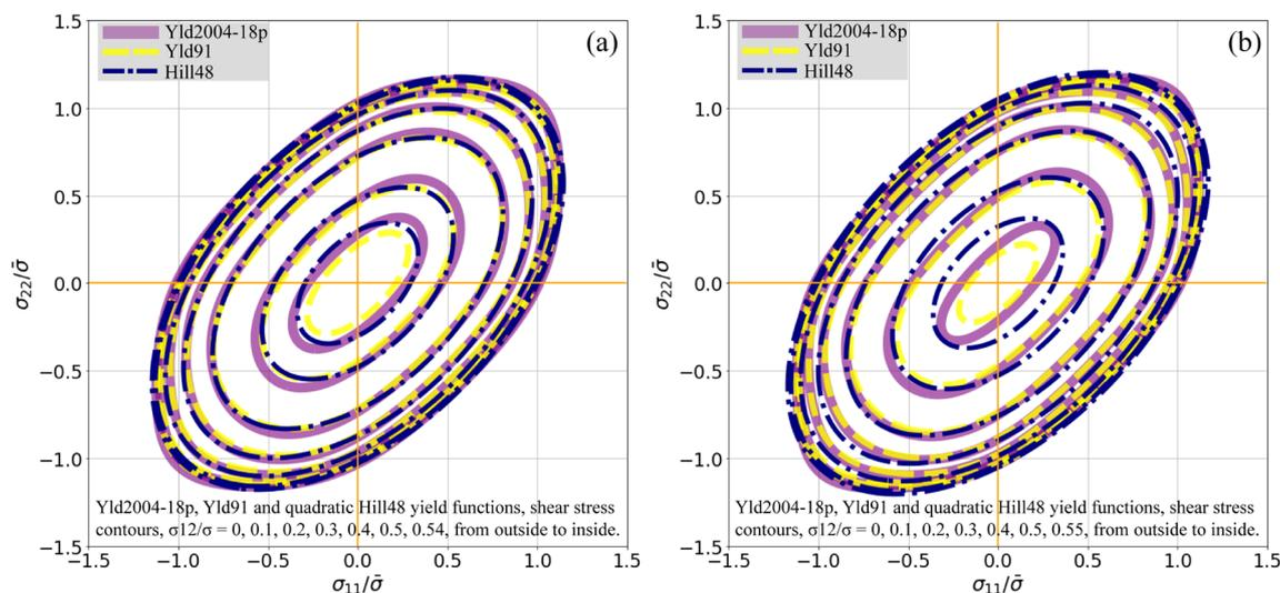
**Figure 7.** Tricomponent  $(\sigma_{11} - \sigma_{22} - \sigma_{12})$  yield loci with constant  $\sigma_{12}/\bar{\sigma}$  contours predicted by the calibrated yield functions for the DP980 sheet. The equivalent deformation stage with the specific plastic work of (a) 3 MPa and (b) 8 MPa.  $\bar{\sigma}$  denotes the uniaxial tensile stress in RD obtained from the VL.
