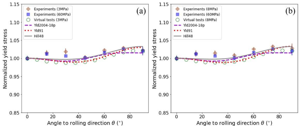
**Figure 9.** Normalized yield stress  $Y_0$  versus  $\theta$  of the DP980 sheet at deformation stages with the specific plastic work of (a) 3 MPa and (b) 8 MPa. The lines are the predicted results of the calibrated yield functions. The diamonds and squares represent experimental values at an interval of 15° from RD to TD and the open circles are the results obtained from virtual tests of uniaxial tension at an interval of 7.5° from RD to TD.
