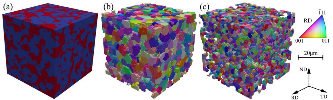
**Figure 1.** (a) The high-resolved dual-phase RVE (DP-RVE) used for CP simulations; red color represents the martensite phase and blue the ferrite. (b) and (c) are the separated ferrite and (c) martensite phases colored with the RD IPF.
