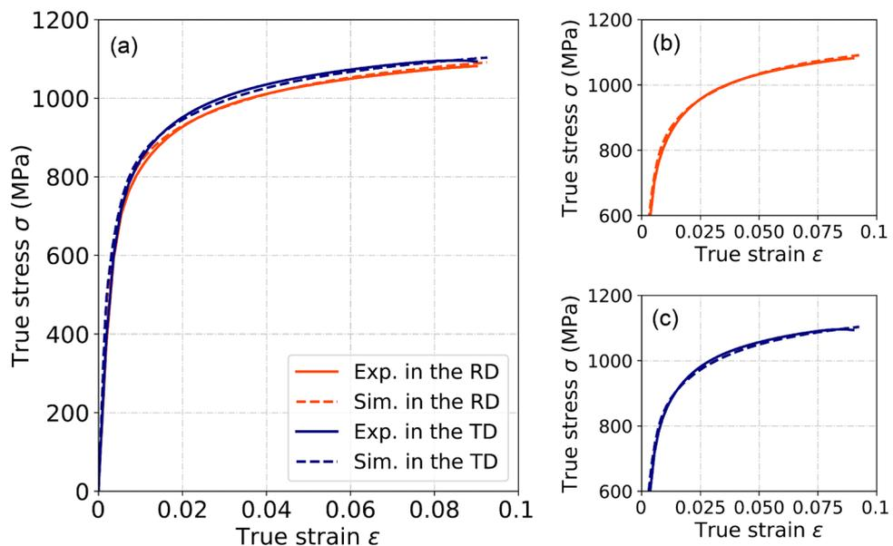
**Figure 3.** (a) Comparison of the flow stress curves predicted the calibrated CP model with the experimental ones along RD and TD. The partial magnifications of the results in RD and TD are shown in subfigures (b) and (c), respectively.
