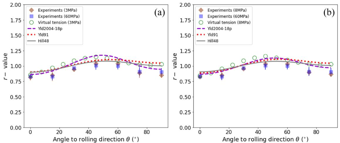
**Figure 8.**  $r$ -value versus  $\theta$  of the DP980 sheet at deformation stages with the specific plastic work of (a) 3 MPa and (b) 8 MPa. The lines are the predicted results of the calibrated yield functions. The diamonds and squares represent experimental values at an interval of 15° from RD to TD and the open circles are the results obtained from virtual tests of uniaxial tension at an interval of 7.5° from RD to TD.
