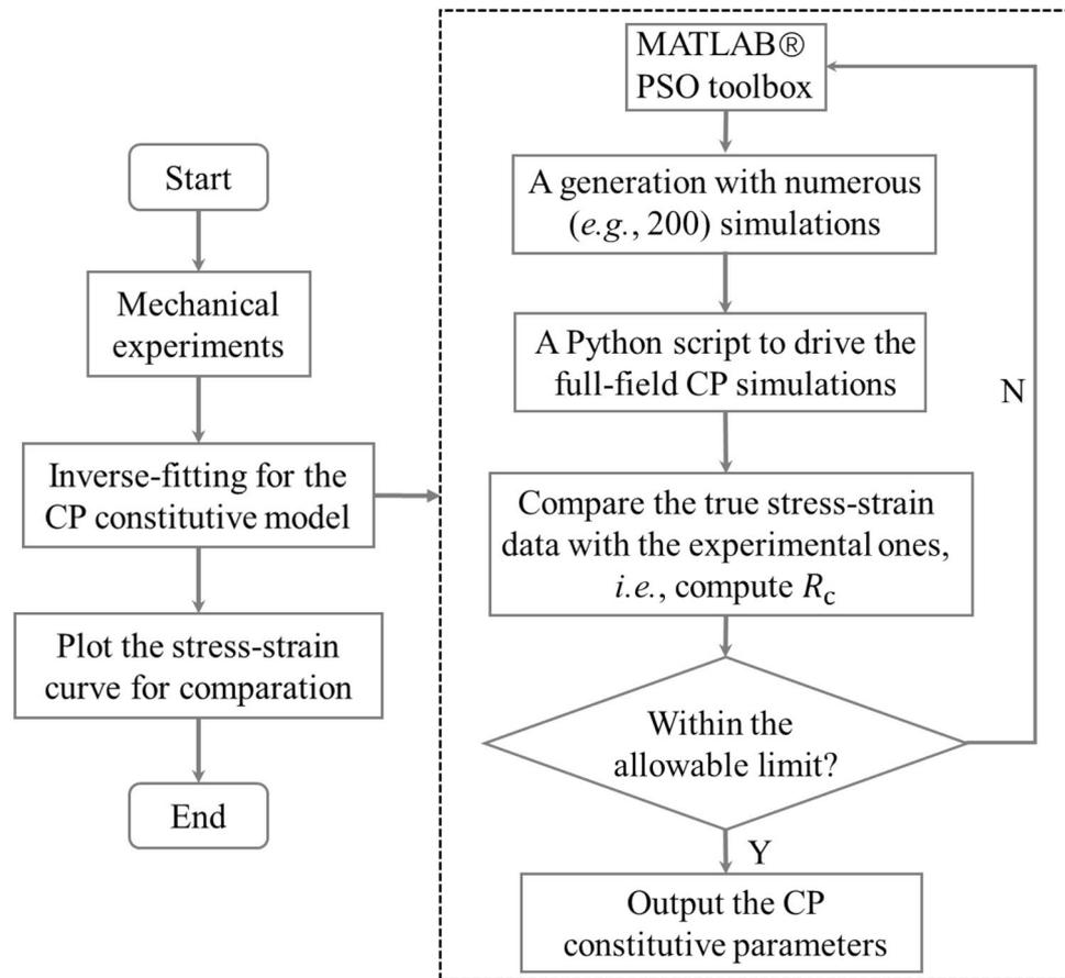
**Figure 2.** The flow chart of the in-house inverse simulation method for identifying the CP model parameters.
