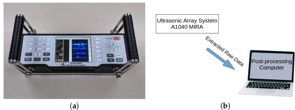
Figure 2. (a) Ultrasonic array system, A1040 MIRA and (b) experiment setup.
