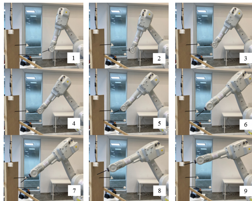
Figure 9. Real-world test: (1) The robot starts moving from the start point (Sphere). (2–8) The robot track the found path while avoiding the obstacle. (9) The robot reaches the target (Cube).
