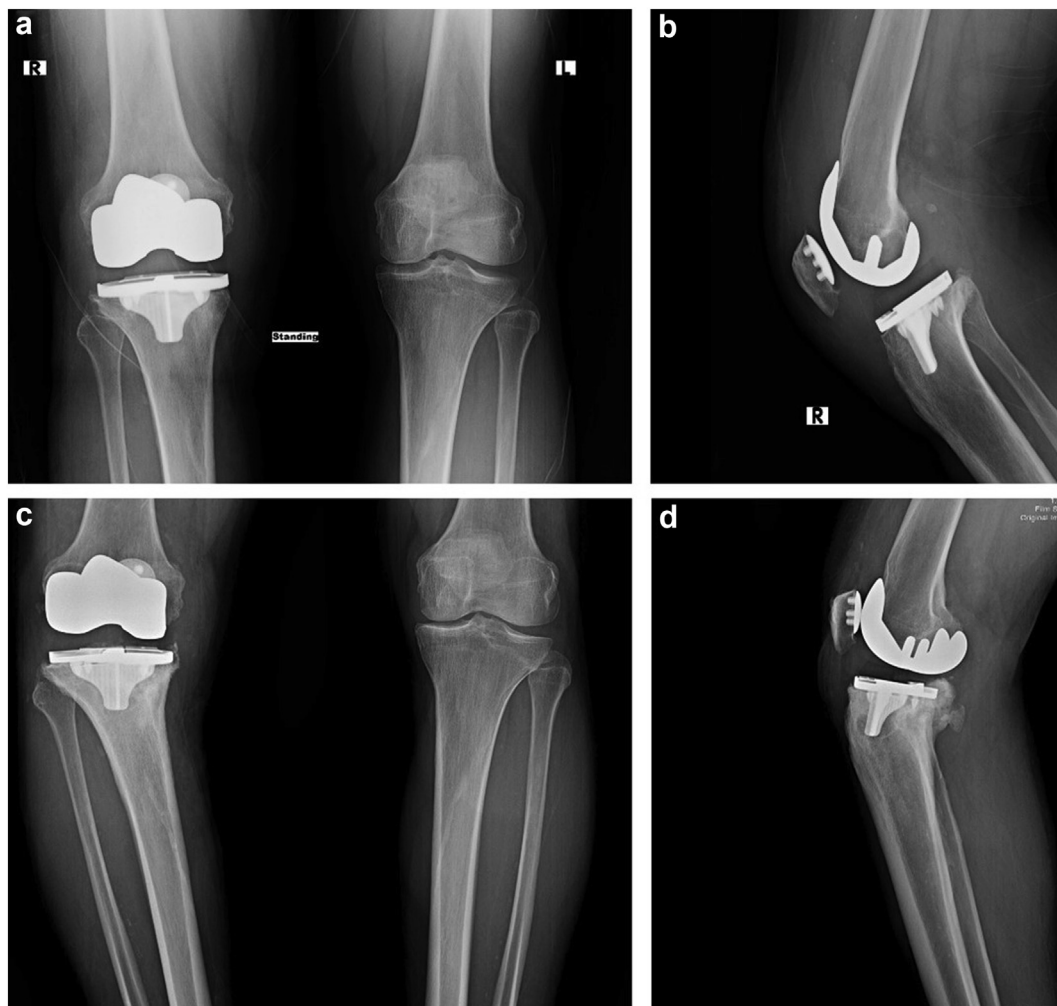
Figure 6. Follow-up radiographs approximately 6 months (a-b) and 4 years (c-d) after index procedure depicting tibial baseplate fracture and posterior subsidence.
