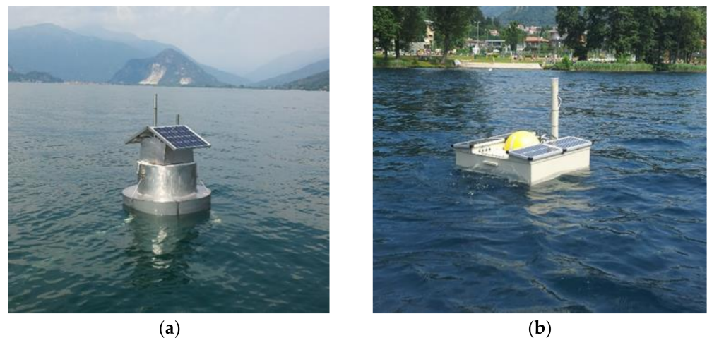
Figure 6. Limnological buoys: (a) fixed buoy on Lake Maggiore; (b) mobile (portable) buoy on Lake Orta.
