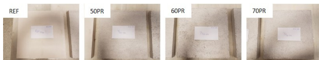
Figure 6. Boards used in the surface thermal comfort test.
