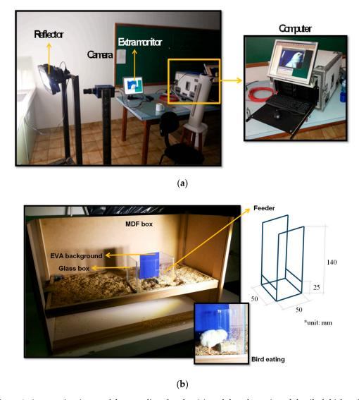
**Figure 1.** An overview image of the recording chamber (a), and the schematic and detail of chick eating at the glass trough inside the recording chamber (b).
