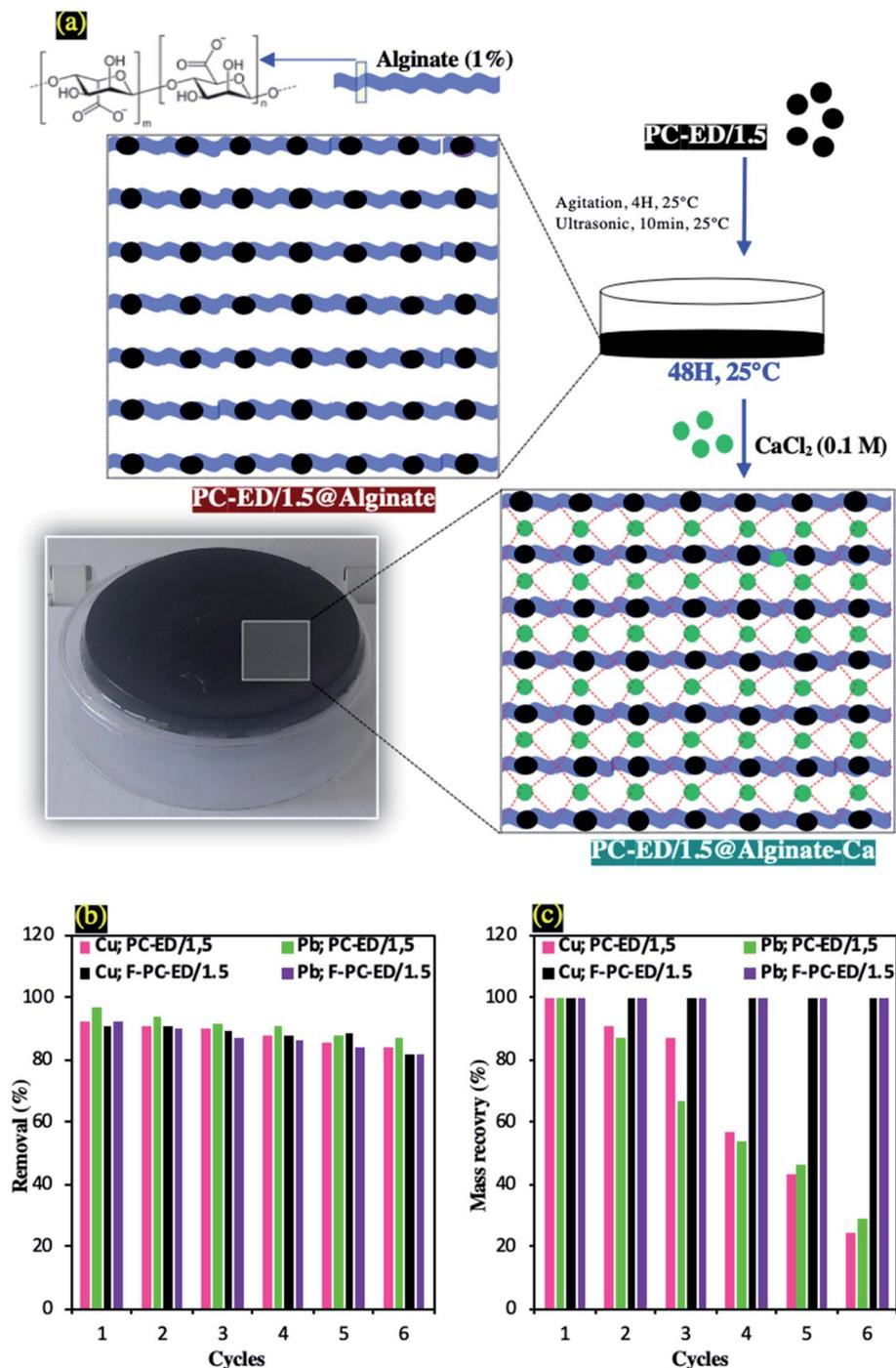
Fig. 9 (a) Protocol of preparation of PC-ED/1.5@alginate-Ca three-dimensional networks, (b) regeneration study and (c) Mass recovery of PC-ED/1.5 and F-PC-ED/1.5.
