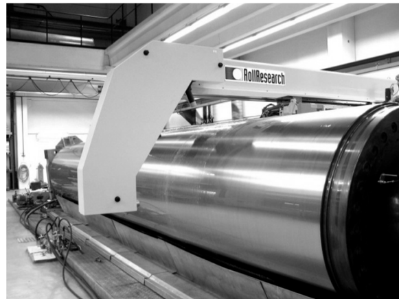
Figure 4. Roll measuring device for measuring the roundness and shape of a roll.
