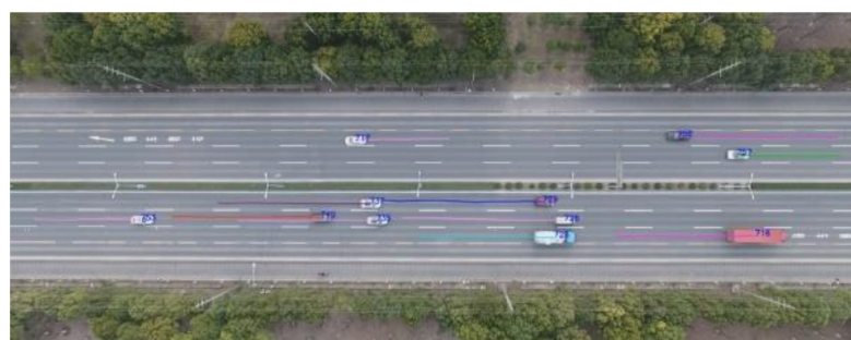
Figure 3. UAV video screenshot of road traffic and trajectory extraction.
