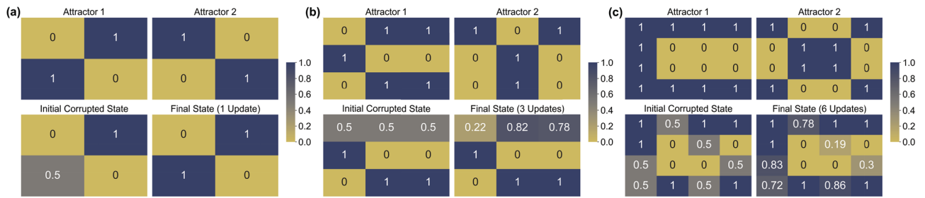
Figure 4. QASM simulation of QHAM of size 4, 9, and 16. Simulation results of the quantum Hopfield associative memory system for sizes (a) 4, (b) 9 and (c) 16 31 with two given attractor states. Each color graded box represents a qubit in each system state, and the number inside the box is the exact probability of measuring |1\rangle for that individual state.
