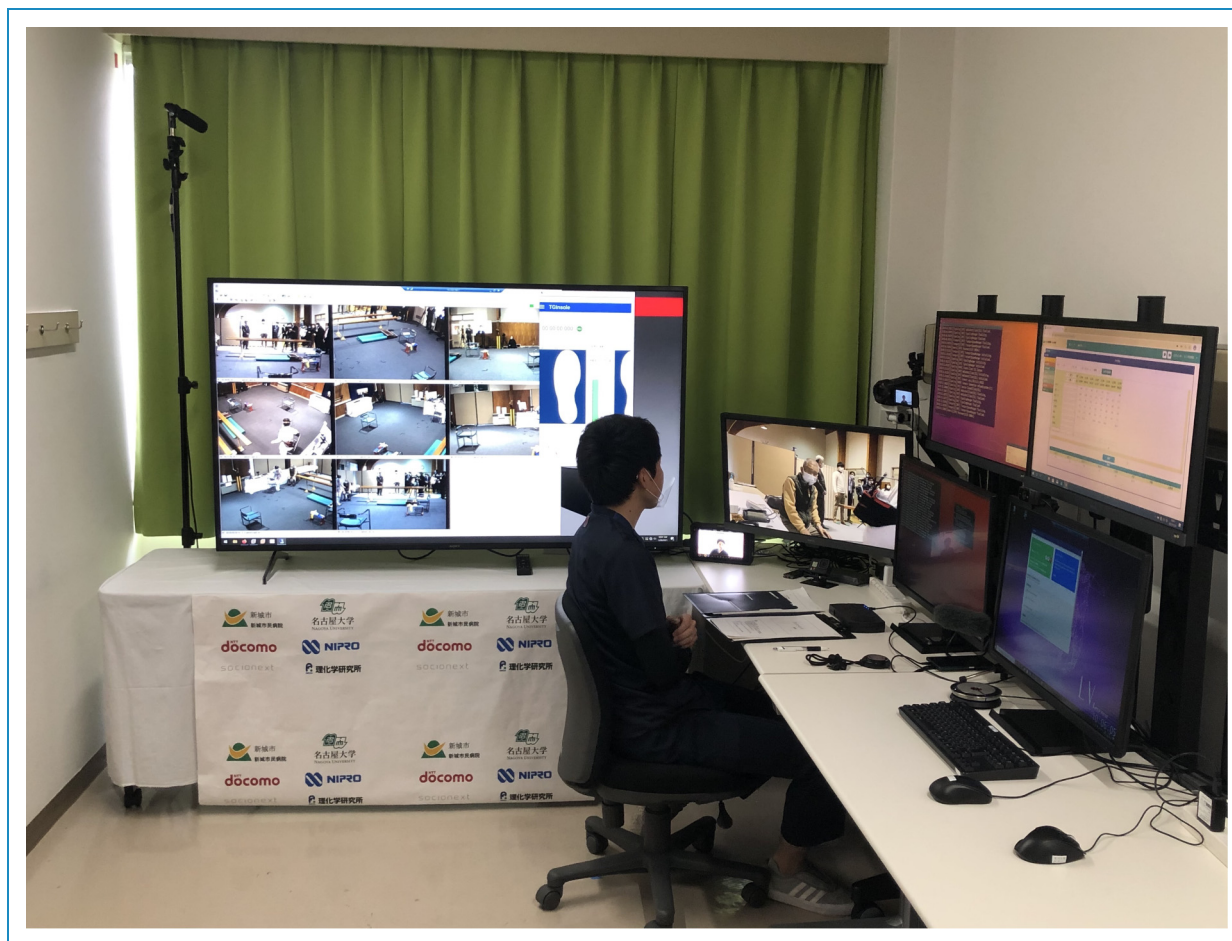
Figure 2. A view of Shinshiro municipal hospital (core hospital). A physical therapist is conducting a medical interview. The motion capture system and dynamic load detected by the insole-type internet of things are shown on a large monitor.
