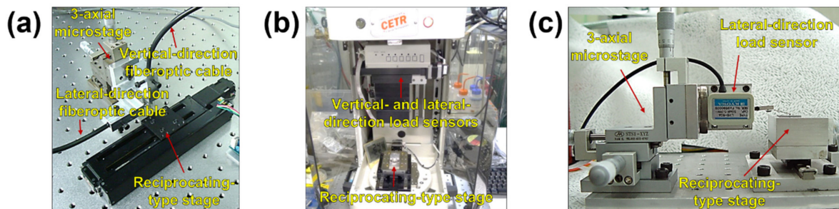
Figure 4. Images of (a) custom-built tribotester with two fiberoptic sensors and a cantilever tip; (b) commercial tribotester (CETR) consisting of two load sensors; (c) Custom-built micro-tribotester comprising a load sensor.
