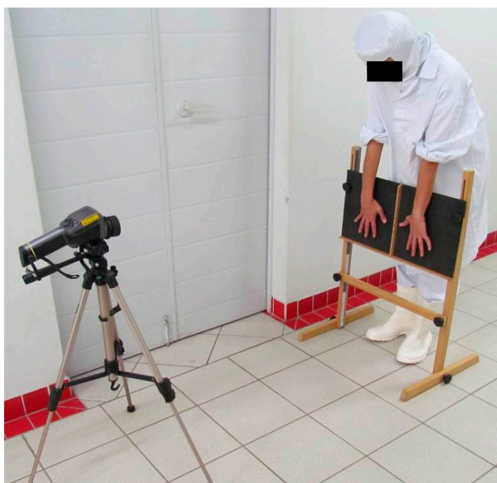
Figure 1. Infrared portable camera and frame for capturing the thermographic images.
