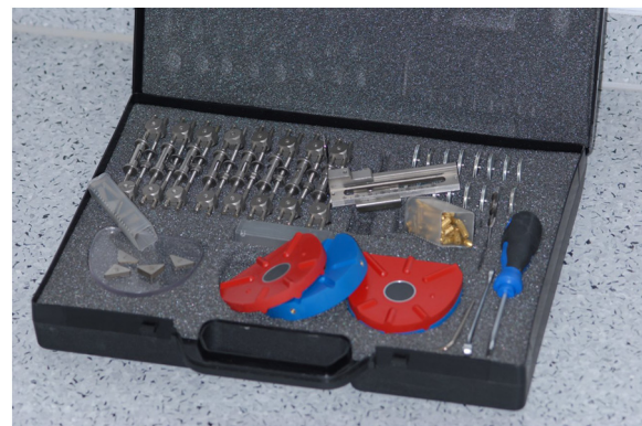
Figure 4 Hardware components of the University Münster Model Surgery System for Orthognathic Surgery (Orbis Will, Ahaus, Germany).
