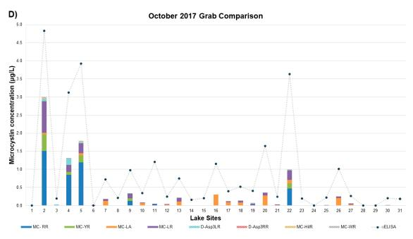
**Figure 3.** 2017 sampling period; (**A**) July, (**B**) August, (**C**) September, and (**D**) October. Data comparison of total MC ( $\mu$ g/L) detected by LC/MS/MS (bars) and Adda-enzyme-linked immunosorbent assay (Adda-ELISA) (dots).
