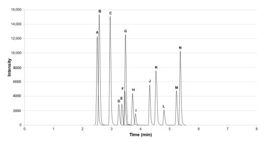
**Figure 2.** Chromatogram of selected microcystins (MCs), nodularin, and surrogate standard (L). A: D-Asp<sup>3</sup>-MC-RR; B: MC-RR; C: Nodularin; D: MC-YR; E: MC-HtyR; F: MC-LR; G: D-Asp<sup>3</sup>-MC-LR; H: MC-HilR; I: MC-WR; J: MC-LY; K: MC-LA; L: C<sub>2</sub>D<sub>5</sub>-MC-LR; M: MC-LW; and N: MC-LF.
