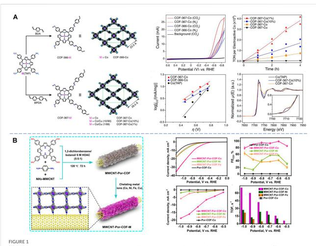
(A) Structures, electrochemical characterizations, and carbon dioxide reduction performance of the metalloporphyrin-derived 2D covalent organic frameworks COF-366-Co and COF-367-Co [reproduced from Lin et al. (2015) with the permission of AAAS]. (B) Design and synthesis of MWCNT-Por-COF-M and its electrochemical characterizations and carbon dioxide reduction performance [reproduced from Dong et al. (2022) with the permission of Elsevier].
