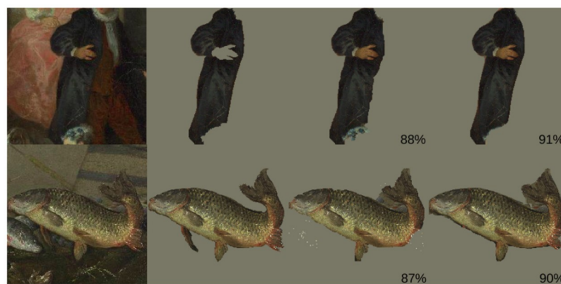
Fig 12. Segmentation visualizations. Left to right: Original Image, Ground Truth Segment, Grabcut Extr Segment, DEXTR COCO Segment. Both Grabcut and DEXTR use extreme points as input. For evaluation, the extreme points are generated synthetically from the ground truth segments. The IOU for each segmentation is shown in the bottom right corner. Top image: Dance before a Fountain , by Nicolas Lancret, 1724, Digital image courtesy of the Getty's Open Content Program. Bottom image: Still life with fish , by Pieter van Noort, 1660, Het Rijksmuseum. Images reproduced under a CC0 license.
