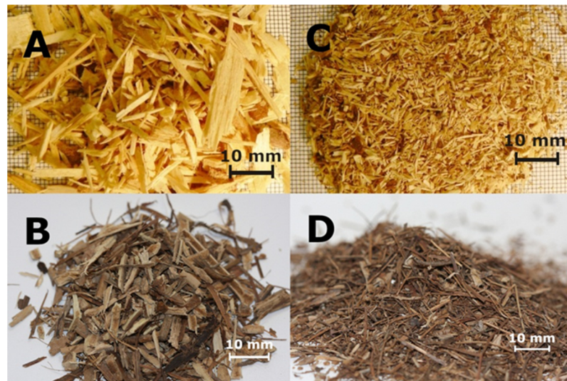
Figure 1. The particles of vine pruning waste: particles for the core layer are (A) pinewood and (B) vine pruning; particles for the face layers are (C) pinewood and (D) vine pruning.
