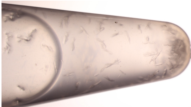
Fig. 4. Spontaneous BRD4(1) crystal formation in reaction tube. BRD4(1) (20 mg/mL in crystallization buffer) crystals grown in a 1.5 mL reaction tube at 12 °C after two weeks.
