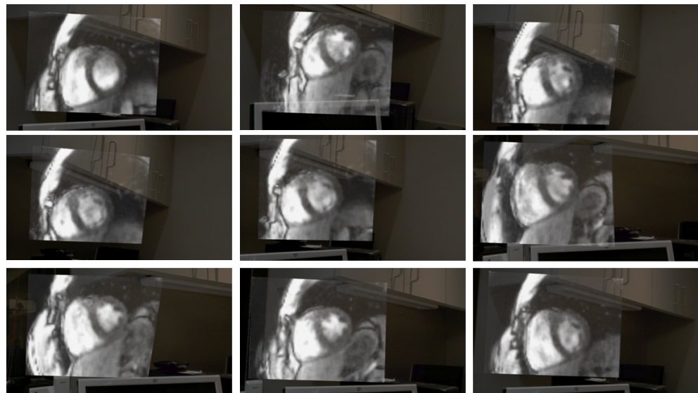
Figure 6. Multiple still frames from a user's perspective of a volumetric scan through a mixed-reality headset are shown. The user moved around the rendering, changed the viewing angle, and moved toward and away from it. The stills were captured by a program in the headset that combines the rendering that is projected to the user with a video capture from the camera embedded in the headset. A video version of this figure is available in the Supplementary Materials.
