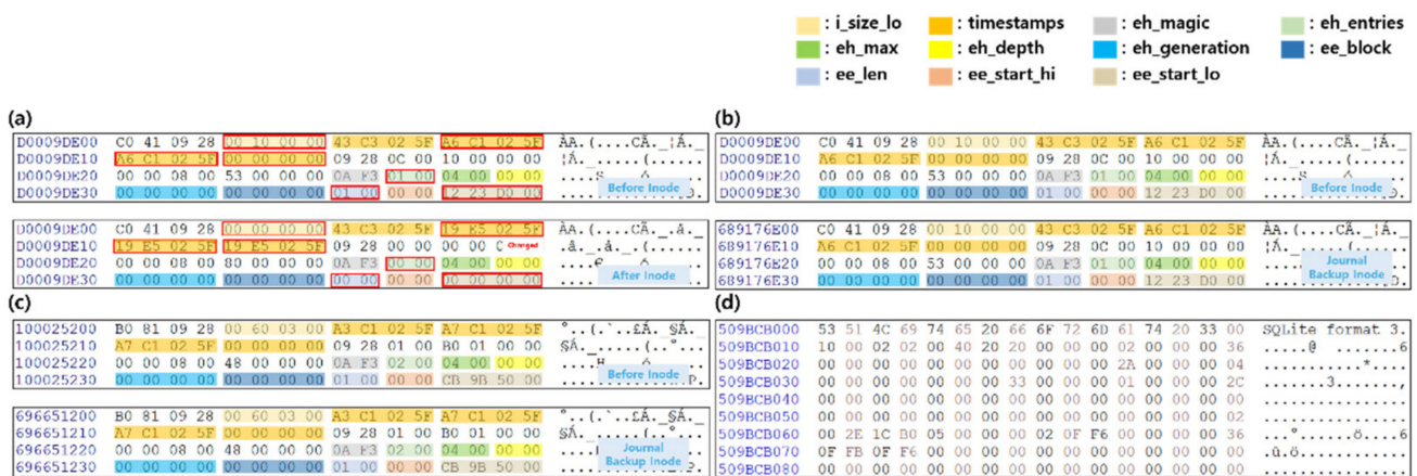
Figure 9. Metadata analysis of filesystem before and after data deletion using scenario III (a) Comparison of /data/data/com.kakao.talk’s directory entries before and after deleting app data (b) Comparison of /data/data/com.kakao.talk’s inode before deletion and journal backup inode (c) Comparison of kakaotalk.db’s inode before deletion and journal backup inode (d) Comparison of kakaotalk.db’s data area found based on journal backup inode. The red box indicates changed fields before and after deletion.
