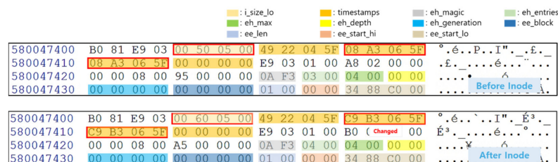
Figure 2. Comparison of mmssms.db’s inode before and after deleting app data using Scenario I. The red box indicates changed fields before and after deletion.
