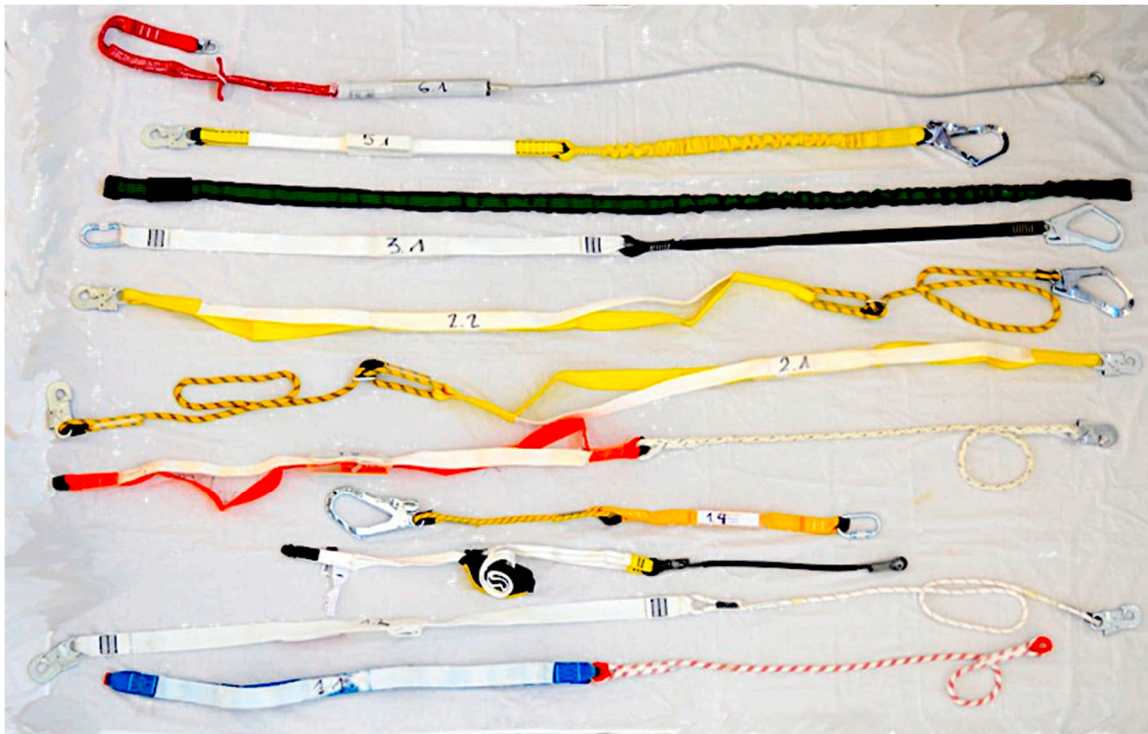
Figure 7. Samples after dynamic performance test.
