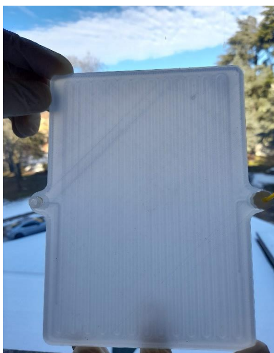
Figure S5. Experimental setup used for photocatalyzed functionalizations under flow conditions: 3D-printed reactor A (top part) and 3D-printed reactor B (bottom part).
