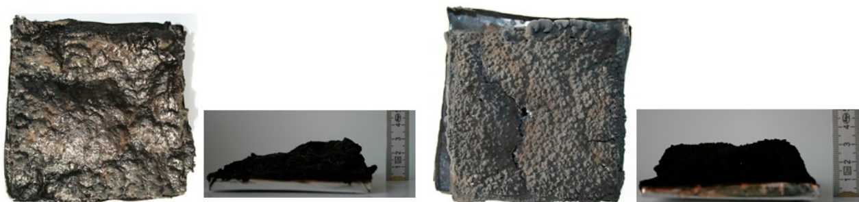
Figure 8. Photographs of the UP/30APP and UP/30LHP after cone calorimetry tests.
