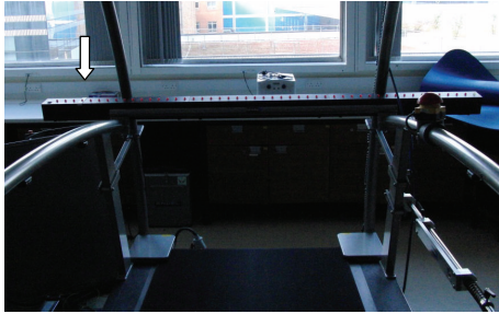
FIGURE 1: Experimental setup of the Bassin Anticipation Timer. Arrow indicates location of the target light with the motion of the stimulus light moving from right to left.
