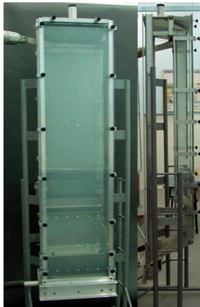
**Figure 3.** Fluidizing column: front view and side view.
