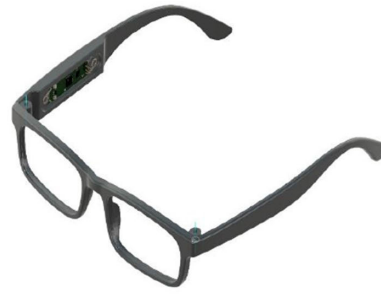
1B. Side arm housing for the electronics board
