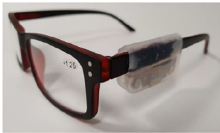
Figure 2. SpecsOn monitor attached to the side arm of the spectacle frame.
