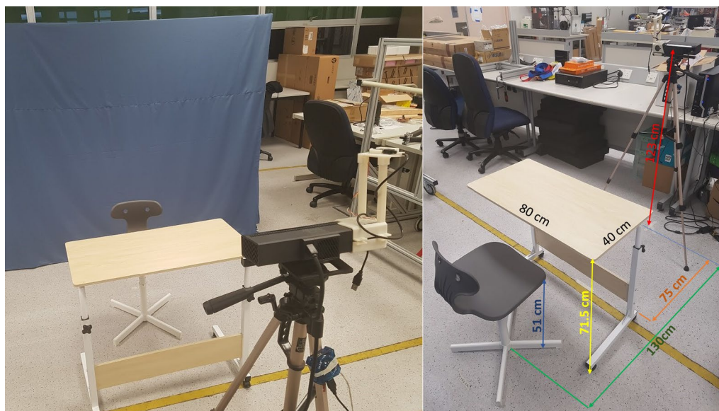
Fig. 2 The table, chair, and the camera setup for Kinect Alone and Kinect+IMU motion capture system. This arrangement is also used in a marker-based motion capture volume to perform simultaneous records from all three motion capture systems
