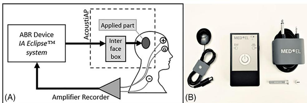
**FIGURE 1** The measurement setup and the AcoustiAP device. The measurement setup (A) shows the ABR system, the AcoustiAP consisting of the interface box and the applied part. The subject with positive (+), negative (–) and ground (G) electrode, connected to the amplifier recorder. A photo of the AcoustiAP device parts (B; image provided by manufacturer). Left to right: The applied part, interface box, cable, magnet door opening tool and a strength three magnet.
