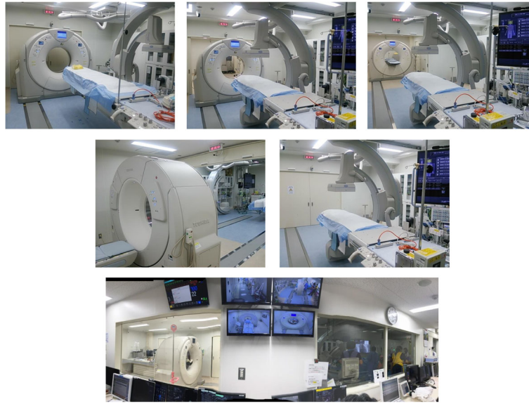
Fig. 2 Photographs showing the dual-room sliding CT scanner system with interventional radiology features. The new CT suite has another radiolucent table. When we perform emergency surgery or interventional radiology for a severely injured or ill patient in the regular emergency room, the sliding CT scanner is moved to the new adjacent CT suite with the radiolucent table, and we can perform CT scanning of another in/outpatient
