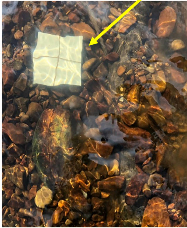
FIG 1 Representative image of the sampling tile (arrowhead in yellow) used for collecting biofilm from the river. The tile was tightly joined to a flat stone by using a thin wire to minimize the outflow.
