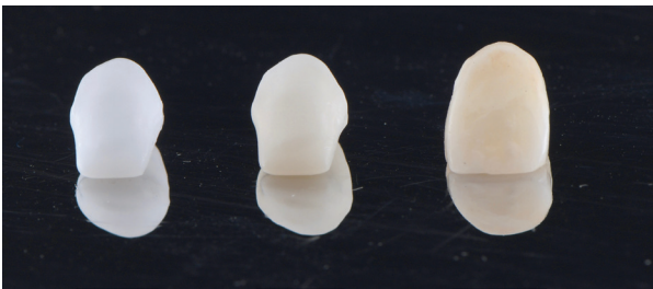
Fig. 2: White Zr core, colored Zr core and ht Zr crowns.
