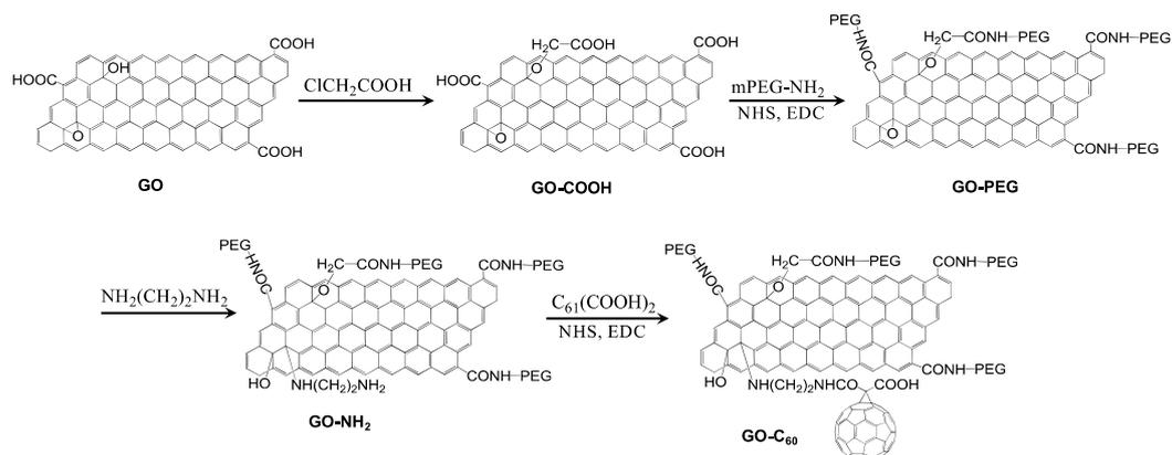
**Figure 11.** Synthesis of GO-C<sub>60</sub>. Image adapted with permission from [157].
