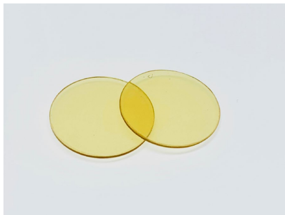
Figure 4. Photograph of compression-molded BP1 sheets used in enzymatic degradation testing.
