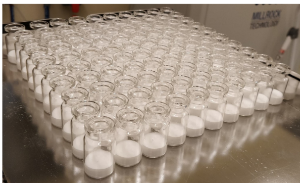
Fig. 4. Photograph of the batch with 3 ml mannitol 5% v/v filled in 6R Schott vials after the microwave-assisted lyophilization cycle (18 GHz, 79 W). There are no signs of product collapse.
