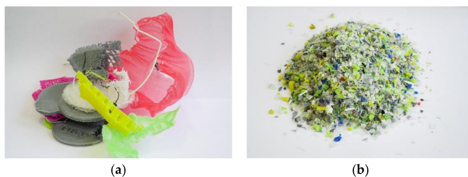
Figure 1. Appearance of polylactide waste: (a) after 3D printing, (b) after grinding.
