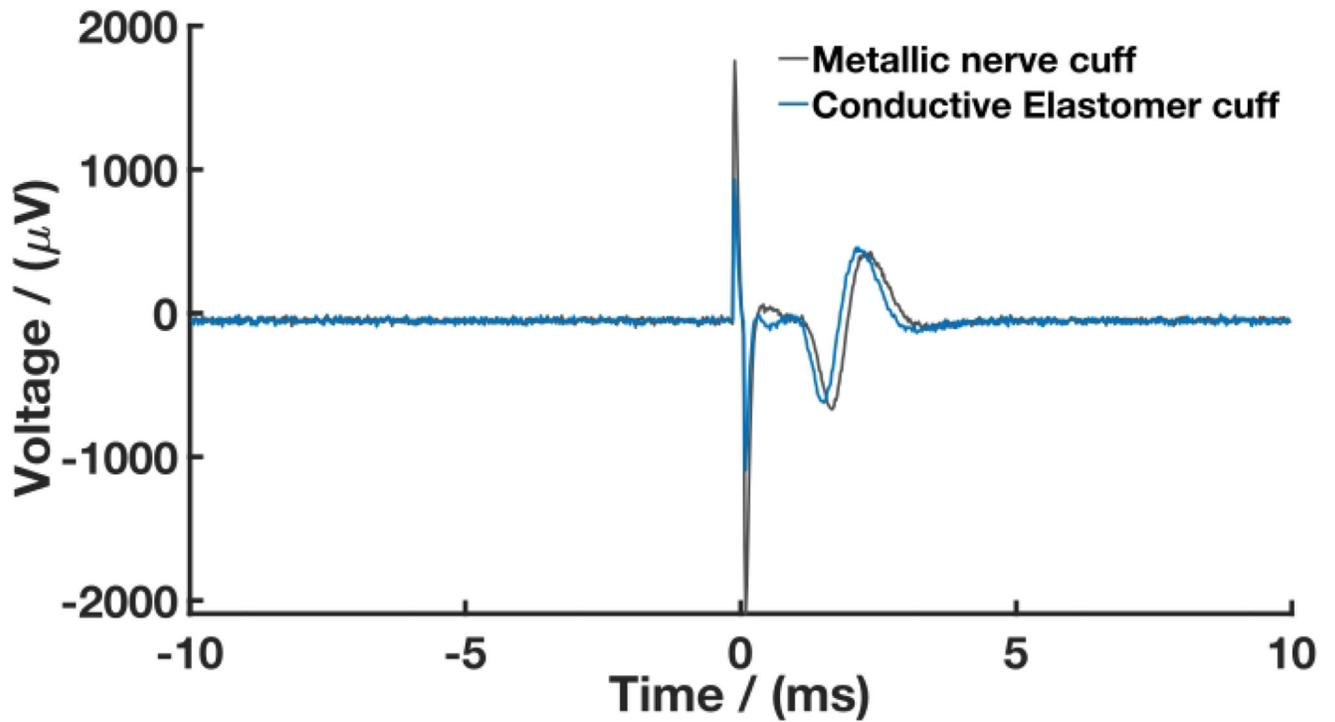
**Figure 2. Representative CAPs obtained *ex vivo* following stimulation by metallic and conductive elastomer nerve cuff arrays.**
