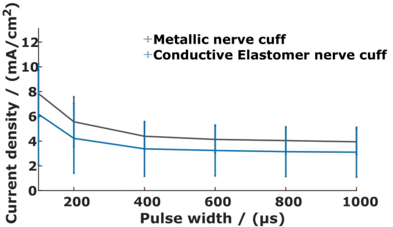
**Figure 3. A-fibre activation threshold of metallic and conductive elastomer cuff arrays.** Error bars represent  $\pm 1$  standard deviation from the mean. Reproduced with modifications from Cuttaz, E. A. et al. (2021)<sup>22</sup>. [Please click here to view a larger version of this figure.](#)
