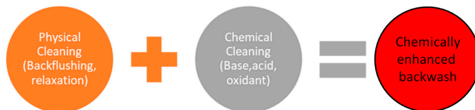
Figure 3. Membrane cleaning methods; physical cleaning, chemical cleaning, and their combination (chemically enhanced backwash).
