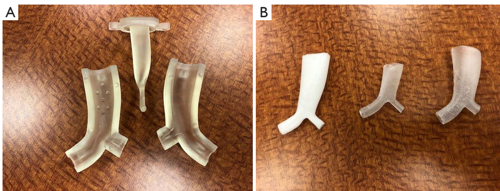
Figure 2 Example of airway stents produced using 3DP technology. A patient's CT scan was imported into 3DP software which was then used to produce a negative mold on a 3D printer (A). Silicone was injected into this mold to produce the final stent product (B). 3DP, three-dimensional printing; CT, computed tomography.
