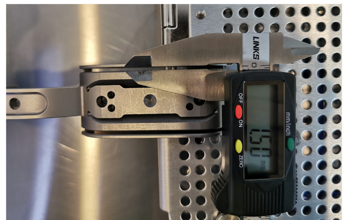
Fig. 6. The thickness of the gap of the cutting jig.
