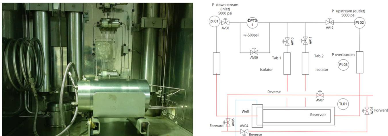
Figure 3. Core flood system (FDS350) apparatus, and piping and setup diagram of the locations of pressure gauges.
