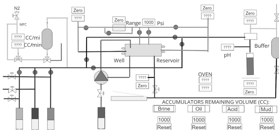
Figure 4. Schematic of formation damage and well treatment services (FDS350).
