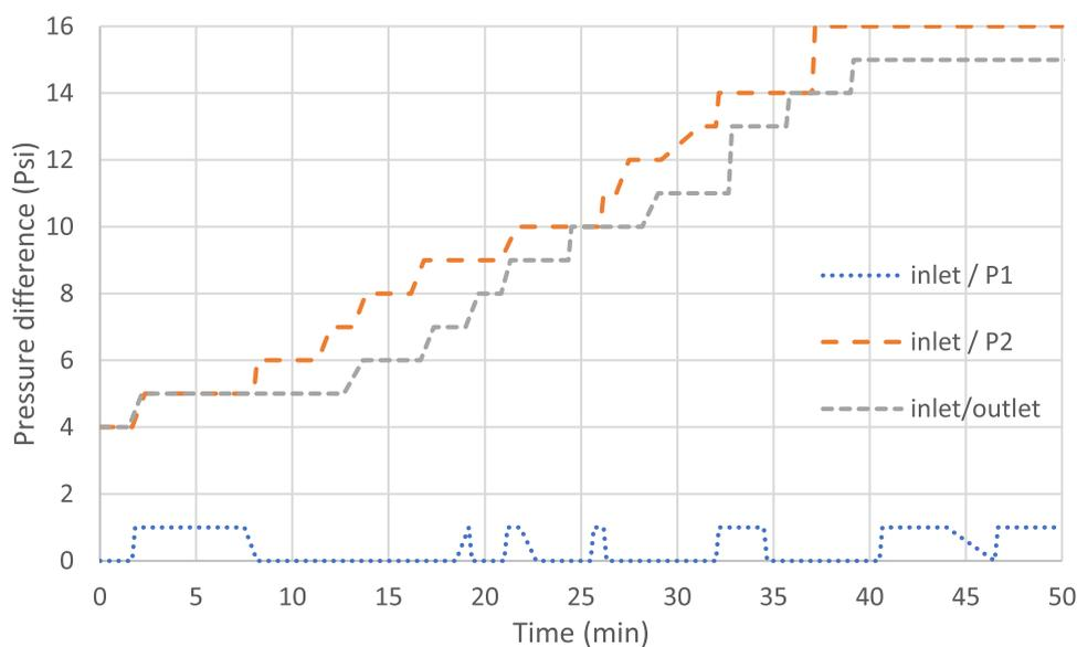
**Figure 8.** Pressure vs time results of the sample with high roughness. (The inlet/outlet line indicates the pressure difference between the two ends of the plug. The inlet/P1 line refers to the pressure difference between the inlet end and Tab1 through the core holder. The inlet/P2 line shows the pressure difference of the inlet end and Tab2 gauge in the middle of the plug in the core holder).
