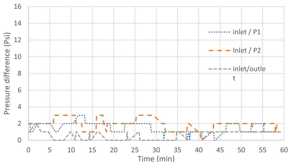
**Figure 6.** Pressure vs time results of the sample with low roughness. (The inlet/outlet line indicates the pressure difference between the two ends of the plug. The inlet/P1 line refers to the pressure difference between the inlet end and Tab1 through the core holder. The inlet/P2 line shows the pressure difference between the inlet end and Tab2 gauge in the middle of the plug in the core holder).
