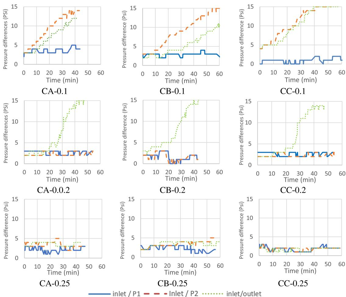
**Figure 5.** Pressure vs time results of sample tests of fluid composition with different fracture widths. (The inlet/outlet line indicates the pressure difference between the two ends of the plug in the core holder. The inlet/P1 line refers to the pressure difference between the inlet end and Tab1 through the core holder. The inlet/P2 line shows the pressure difference between the inlet end and Tab2 gauge in the middle of the plug in the core holder).
