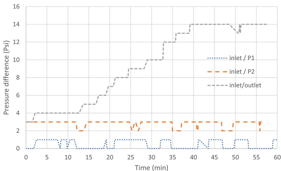
**Figure 7.** Pressure vs time results of the sample with medium roughness. (The inlet/outlet line indicates the pressure difference between the two ends of the plug. The inlet/P1 line refers to the pressure difference between the inlet end and Tab1 through the core holder. The inlet/P2 line shows the pressure difference between the inlet end and Tab2 gauge in the middle of the plug in the core holder).
