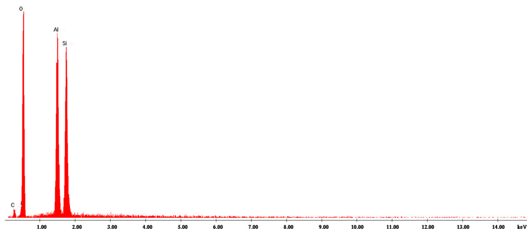
Figure 3. The EDX result of Hal-SWCNT 96:4-350.
